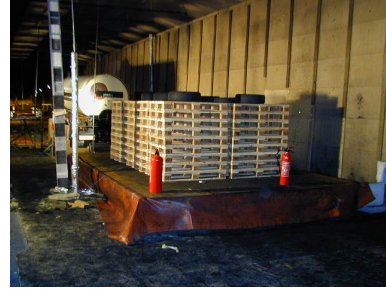
72 wood cribs and tanker on short distance
