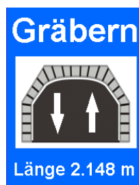
Figure 3: Example of application of the “tunnel sign”
