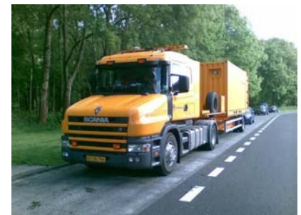
Foto: RTV Drenthe De Deense High Speed Deflectometer
